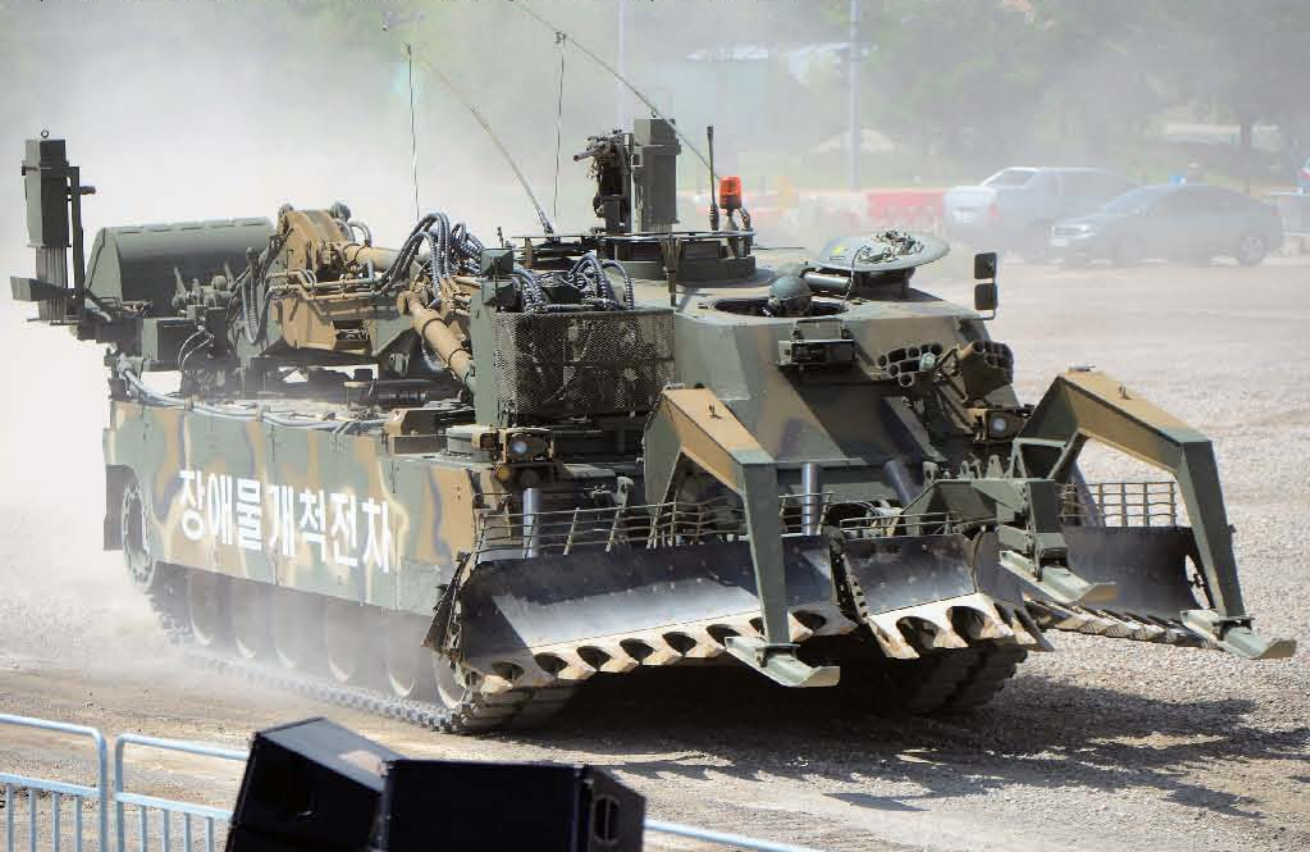
Hyundai Rotem's Obstacle Tank which has been approved for service in July 2018. It is specialized for anti-mine operation.
