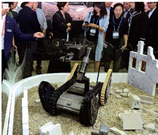
3 Hanwha Land Systems introduced all-terrain unmanned vehicle which can operate in dangerous and hostile areas for reconnaissance and transportation of cargos 160kg. Soldier could operate the unmanned vehicle via monitor from 1km distance and it can transmit communication from air drones and other assets as well. Through deep learning technology, UAV can identify persons and vehicles as well. Equipment attached the rear of the vehicle, which looks like many poles in shape of microphone, is sniper detection system. Introduced by Zain Technology, it can be used to detect enemy's gunshot fire and locate the hostile.
