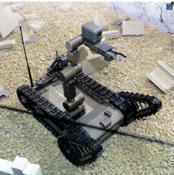
3 Hanwha Land Systems introduced all-terrain unmanned vehicle which can operate in dangerous and hostile areas for reconnaissance and transportation of cargos 160kg. Soldier could operate the unmanned vehicle via monitor from 1km distance and it can transmit communication from air drones and other assets as well. Through deep learning technology, UAV can identify persons and vehicles as well. Equipment attached the rear of the vehicle, which looks like many poles in shape of microphone, is sniper detection system. Introduced by Zain Technology, it can be used to detect enemy's gunshot fire and locate the hostile.
