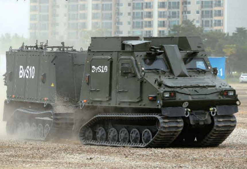
All-terrain BvS10 can transport troops or deliver cargo in any areas and weather conditions. Mountainous and rocky terrain to snow and muddy areas, BvS10 is also amphibious capable and carry up to 5 tons of cargo.
