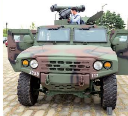
LIG Nex1's Hyungung guided missile installed on Kia Motor's KLTV. Hyungung has fire and forget system to increase shooter's survivability and has very effective armor piercing and firing range distance compared to other guided anti-tank missiles. There are several variations available such as infantry version and mounted versions.
